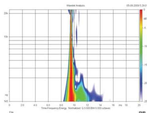
Figure 20 - Wavelet analysis of the time impulse response shows very low amount of internal reflection
