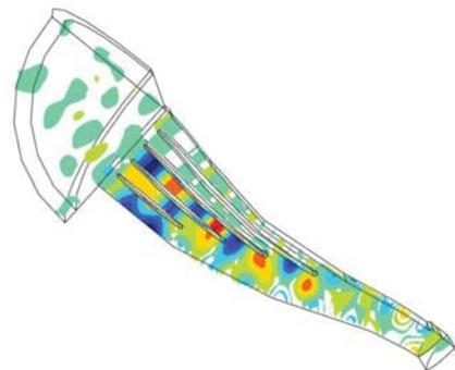
Figure 38 - Computer simulation of inner wave front propagation at 16 kHz where source is a convex dome
