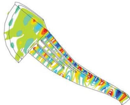
Figure 37 - Computer simulation of inner wave front propagation at 12.5 kHz where source is a convex dome
