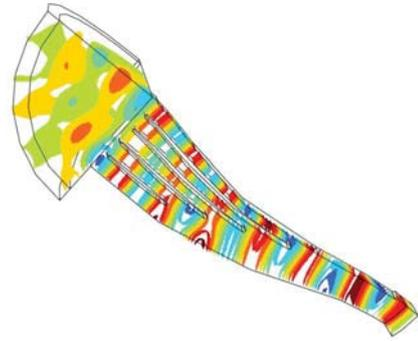
Figure 36 - Computer simulation of inner wave front propagation at 10 kHz where source is a convex dome
