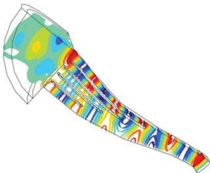
Figure 35 - Computer simulation of inner wave front propagation at 8 kHz where source is a convex dome
