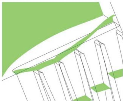
Figure 40 - Wave front shape calculated at the waveguide exit at 5 kHz. Driving source: convex dome
