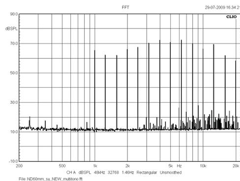
Figure 19 - Multitone analysis from 1 kHz to 20 kHz
