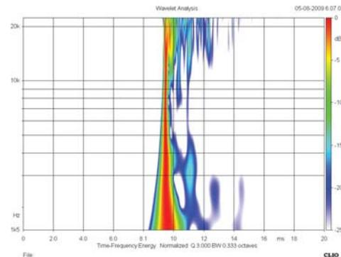
Figure 22 – Wavelet analysis for the alternative HF driver. It can be seen the effect of HF bouncing within the driver itself.
