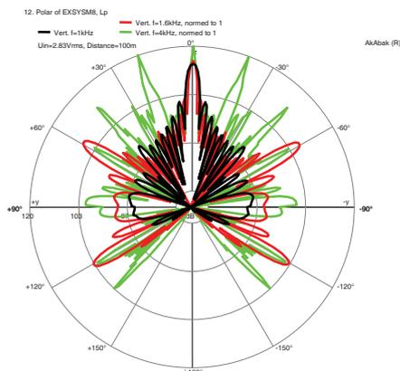
Figure 4 – Polar pattern from an array of loudspeaker units working at frequencies *over* the maximum frequency limit.
