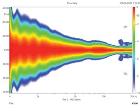
Figure 21 - Polar Directivity Map obtained from the waveguide. First relevant side lobes start to appear at 18 kHz and over
