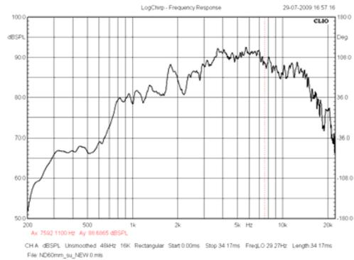
Figure 18 - Frequency response of the waveguide in anechoic chamber
