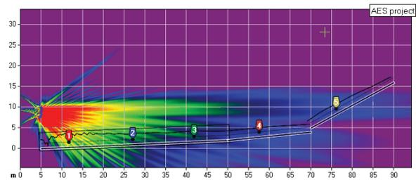
Figure 10 - Vertical dispersion obtained from the curved vertical array
