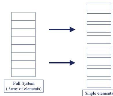
Figure 2 – New design approach: designing an array like if it was a single big speaker and then divide it in modules
