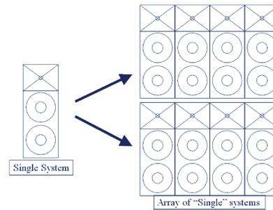
Figure 1 - Traditional array design with a bottom up approach. Design of a loudspeaker system and arraying it in multiple units
