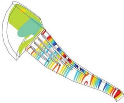
Figure 33 - Computer simulation of inner wave front propagation at 5 kHz where source is a convex dome
