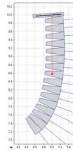
Figure 8 - Proper array curvature to address the vertical coverage requirement into the arena example
