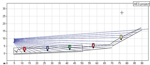
Figure 9 - Vertical system configuration relative to the arena example
