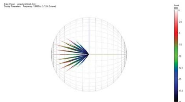
Figure 28 - Array beam at 18 kHz, the HF limit for this waveguide. Expected side lobes and instability can be clearly seen. The use of a better controlled HF driver could greatly improve this behavior.
