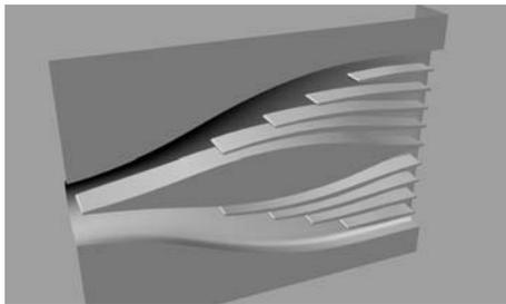
Figure 17 - A 3D model of the inner arrangement of the waveguide
