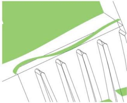
Figure 39 – Wave front shape calculated at the waveguide exit at 5 kHz. Driving source: convex dome
