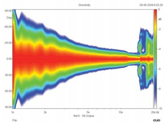
Figure 23 - Directivity polar map measured with the alternative HF compression driver. It can be seen like the HF behavior is heavily affecting also the vertical directivity performances
