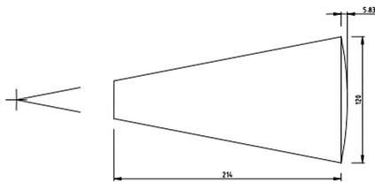
Figure 14 - Reference view of the external dimension of waveguide
