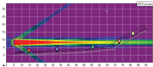
Figure 7 - Vertical dispersion obtained from a straight array calculated for the vocal range. It is not suitable to be applied to the arena example.
