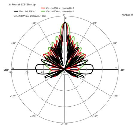
Figure 3 – Polar pattern from an array of loudspeaker units working at frequencies below the maximum frequency limit.
