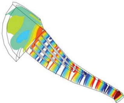
Figure 34 - Computer simulation of inner wave front propagation at 6.3 kHz where source is a convex dome
