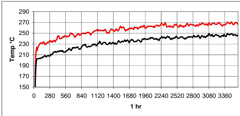
Fig 6 – First hour results of the same AES standard power test (temperature versus time, 15 inch speaker comparison); black plot ISV, red plot external coil.
